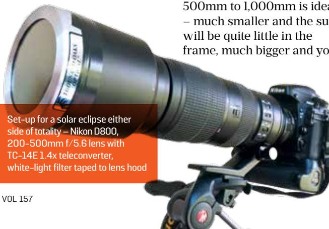
Set-up for a solar eclipse either side of totality – Nikon D800, 200–500mm f/5.6 lens with TC-14E 1.4x teleconverter, white-light filter taped to lens hood
